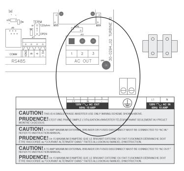
Figure 2.10 AC Output Current Rating Diagram
